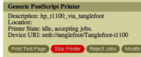
You can print a test page to the Windows printer. This will determine if you have a valid connection from the Mac to the Windows device. You should see the test job appear in the windows print spooler.
